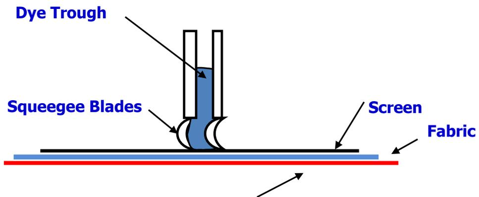
Remember, there is one screen for each color in the pattern. The screens are raised, the blanket precisely moves the fabric to the next color, and the process is repeated. Once each color has been applied, the fabric is removed from the blanket and then processed through the required fixation process. The rubber
